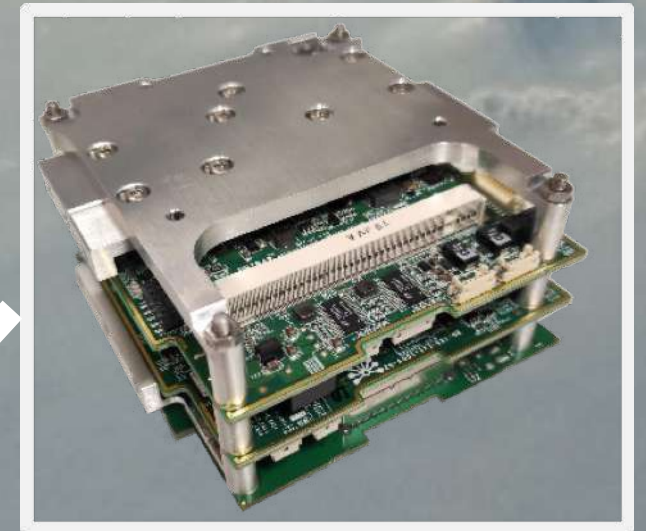
Nebula payload On-orbit Cloud Computing Node (UNIBAP SpaceCloud)
